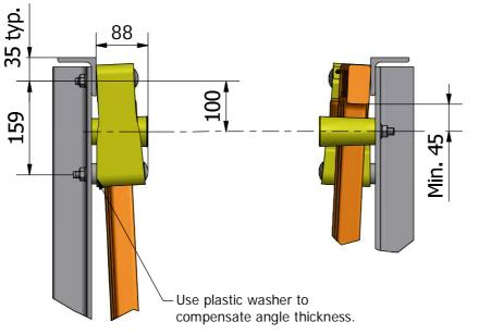
Support block is mounted below the top rail of gate to prevent vertical deflection. IT SHOULD NOT MAKE CONTACT WITH THE GATE OR INTERFERE WITH IT SWINGING CLOSED. Field installations: simply mount the block at least 45mm BELOW the closed bar.
