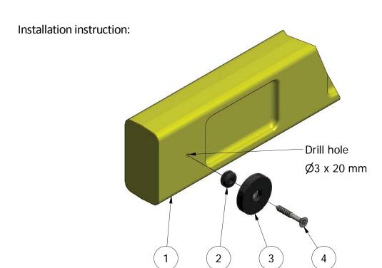
Tighten the screw so far that there is about 5 mm space between the magnet and the safety bar. The rubber washer is provided to secure the magnetic disk, but still allow the disk to be free to "float" or "wobble". In this way, the magnetic disk can make good flat contact with the metal guardrail post.
